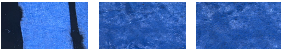
Fig. 9 – TF10E, laser cleaning regime: 1064 nm, F = 0.37 \text{ J/cm}^2 , (left–25×, mid–50×, c. right–100×).
