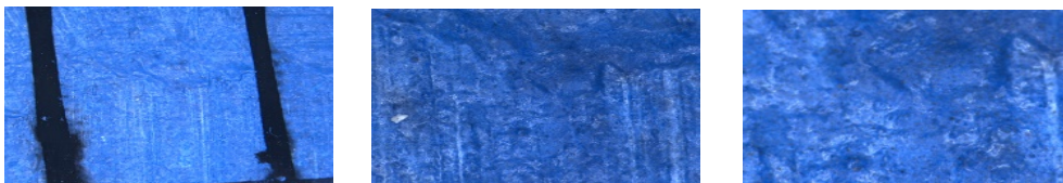
Fig. 10 – TF10F, laser cleaning regime: 1064 nm, F = 0.46 \text{ J/cm}^2 , (left–25×, mid–50×, c. right–100×).
