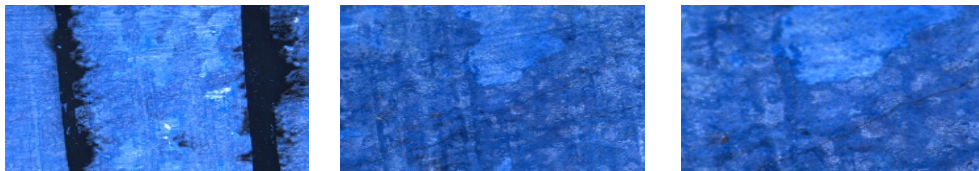
Fig. 7 – TF10C, laser cleaning regime: 532 nm, F = 0.28 \text{ J/cm}^2 (left–25×, mid–50×, c. right–100×).
