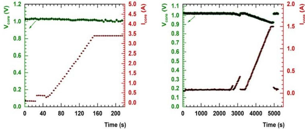
Fig. 1 – (Color on-line) Core current increasing during exposure in  $^{19}\text{F}$  beam (left side) and  $^{22}\text{Ne}$  beam (right side). The saturation in DUT power consumption corresponds to loss of device functionality due to CRAM corruption.
