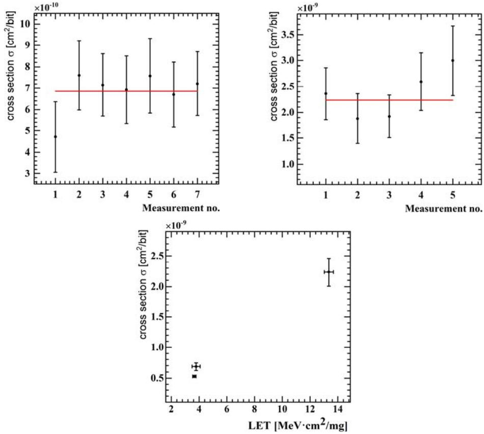
Fig. 3 – (Color on-line) The cross-section measurements for SEU per CRAM bit in <sup>16</sup>O (top left), <sup>28</sup>Si (top right) ion beams. The bottom plot shows the cross-section values with respect to LET for <sup>16</sup>O, <sup>28</sup>Si and <sup>22</sup>Ne.
