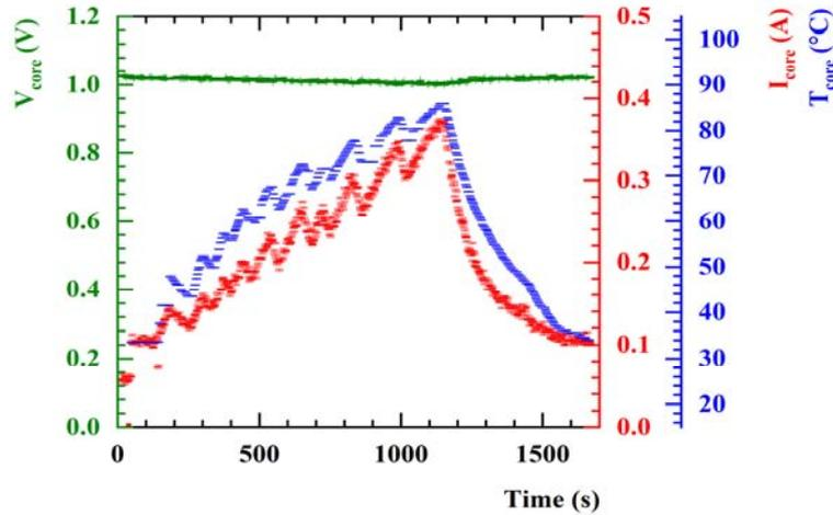
Fig. 2 – (Color on-line) Kintex-7 core current consumption versus its dice temperature.
