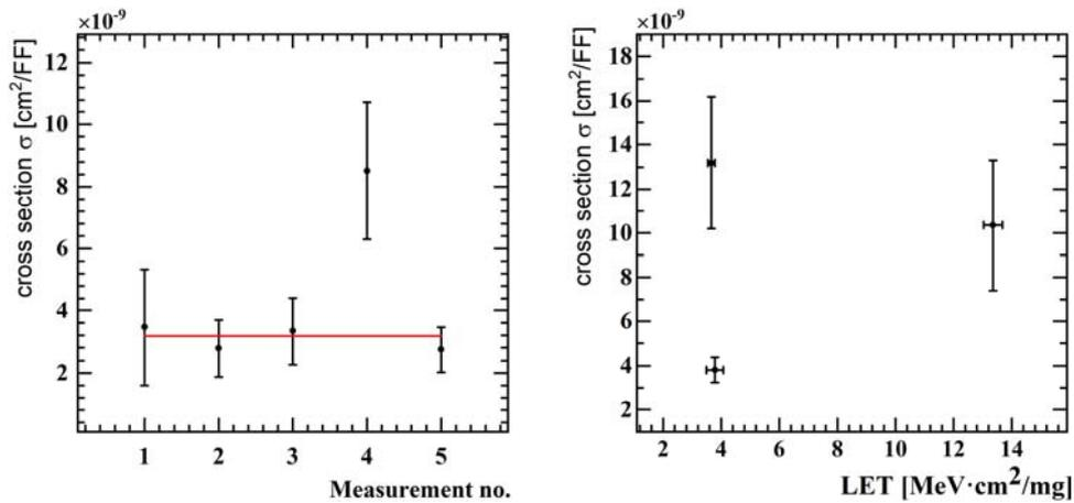
Fig. 5 – (Color on-line) The cross-section measurements for SEU FF in  $^{16}\text{O}$  (left side), while the right-side plot shows the cross-section values with respect to LET for  $^{16}\text{O}$ ,  $^{28}\text{Si}$  and  $^{22}\text{Ne}$ .
