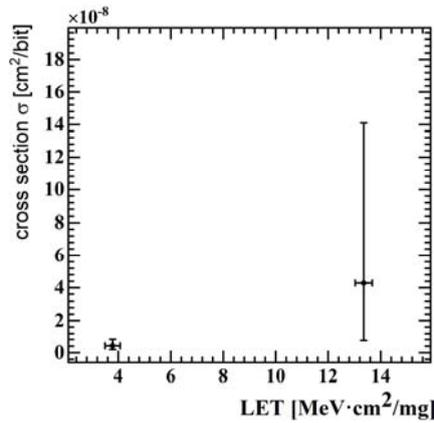
Fig. 4 – Cross-section per BRAM bit versus LET.
