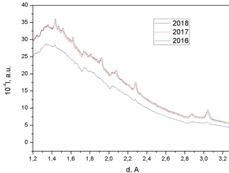
Fig. 5 – Neutron diffraction pattern for the sample composed of CEM III + H<sub>2</sub>O + Al (powder) + Al<sub>2</sub>(SO<sub>4</sub>)<sub>3</sub> + C<sub>6</sub>H<sub>8</sub>O<sub>7</sub> + Pantarhol + LiNO<sub>3</sub>. The sample is prepared at March, 2015.
