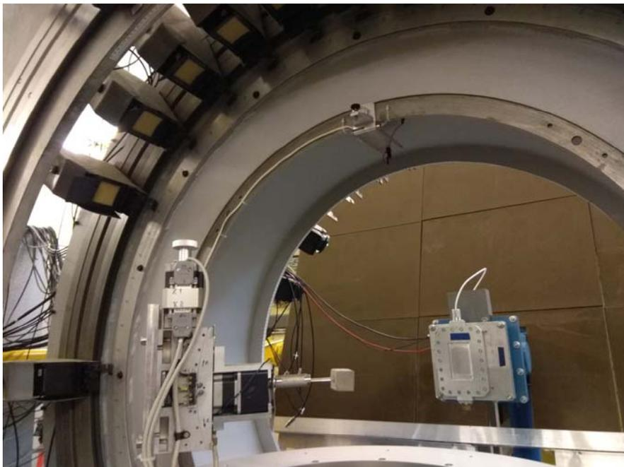
Fig. 1 – The image of SKAT diffractometer – the sample support inside the detector system.
