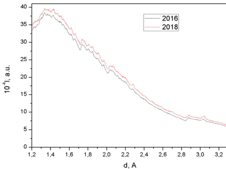
Fig. 4 – Neutron diffraction pattern for the sample composed of CEM III + H<sub>2</sub>O + Al (powder) + Al<sub>2</sub>(SO<sub>4</sub>)<sub>3</sub> + C<sub>6</sub>H<sub>8</sub>O<sub>7</sub> + Pantarhol. The sample was prepared on March, 2015.
