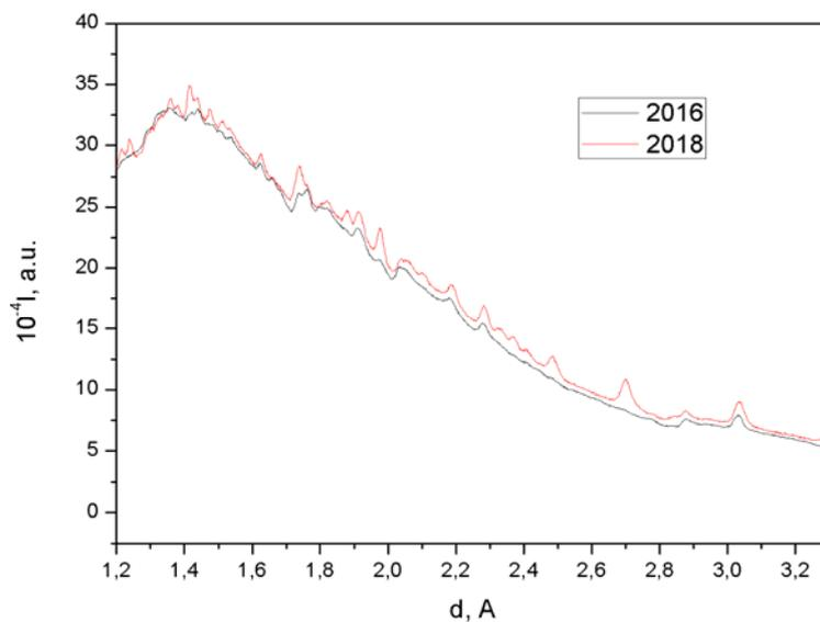
Fig. 3 – Neutron diffraction pattern for the sample composed of CEM III + H<sub>2</sub>O + Al powder. The sample is prepared at March, 2015.
