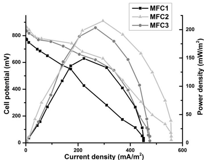
Fig. 5 – Power output and polarization curves of MFC1, MFC2 and MFC3.
