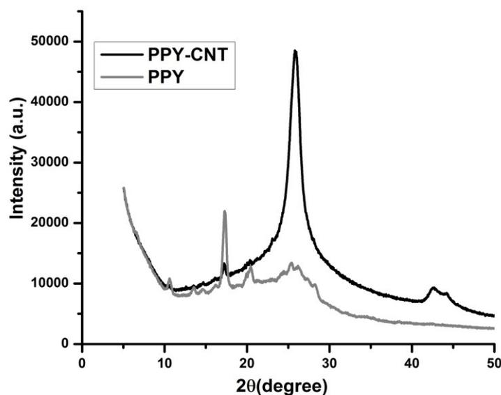
Fig. 4 – X-ray diffraction patterns of PPY and PPY-CNT.
