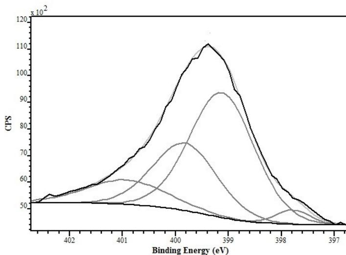
Fig. 1 – N1s core-level spectra of PANI-CNT.
