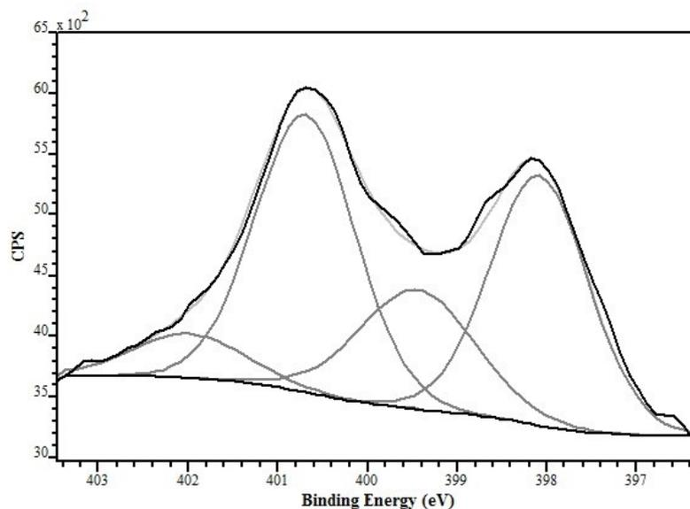
Fig. 2 – N 1s core-level spectra of PPY-CNT.
