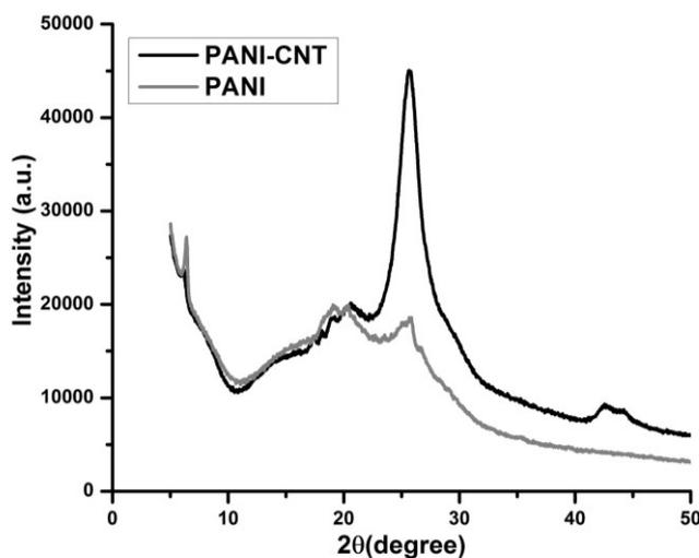
Fig. 3 – X-ray diffraction patterns of PANI and PANI-CNT.
