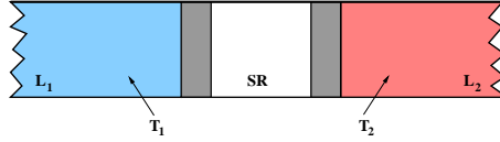
Fig. 1 – Schematic representation of the two-dimensional system composed by the two leads and the scattering region SR. The gray areas are potential barriers which describe the couplings between SR and the two leads L_{1,2} which have different temperatures, T_2 > T_1 .
