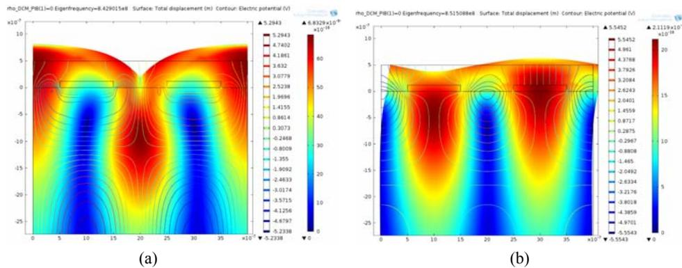
Fig. 4 – Total displacement (color) and electric potential (contour curve) of SAW structure B with  $h_{\text{IDT}} = 120$  nm at: a) resonance frequency (842.9 MHz) and b) anti-resonance frequency (851.51 MHz).
