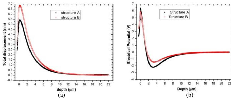
Fig. 6 – Variation of total displacement (a) and electrical potential (b) for SAW structures A and B at resonance frequency as a function of depth.
