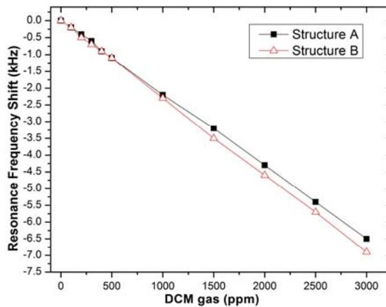
Fig. 8 – Dependence of the resonance frequency shift on the DCM gas concentration for SAW structure A and B.
