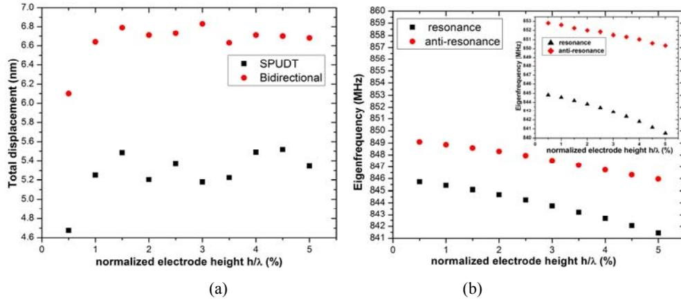
Fig. 3 – The variation of total displacement of SAW structure with bidirectional and SPUDT electrode configurations (a) and frequency edges of the stop band (b) for the parameter sweep of the electrode height. The inset graph from fig. 3.b represents bidirectional configuration response and the other one is referring to SPUDT geometry.
