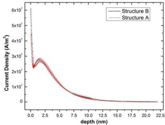
Fig. 7 – Variation of current density for SAW structures A and B at resonance frequency as a function of depth.
