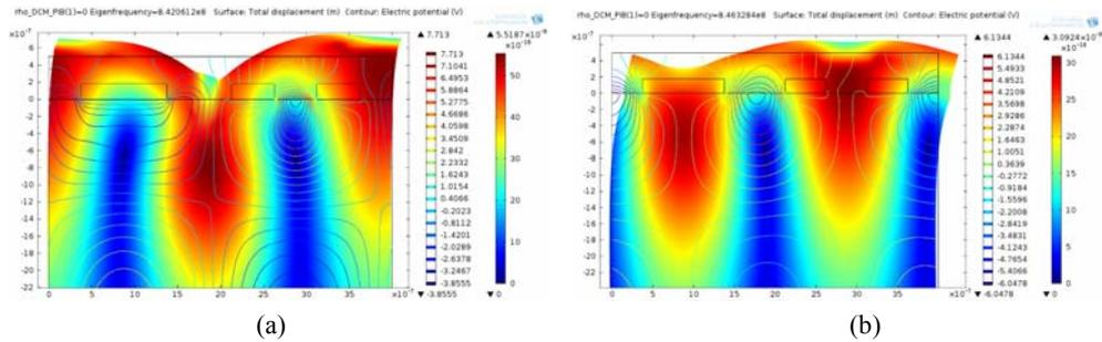
Fig. 5 – Total displacement (color) and electric potential (contour curve) of SAW structure A with  $h_{\text{IDT}} = 180$  nm at: a) resonance frequency (842.9 MHz) and b) anti-resonance frequency (851.51 MHz).
