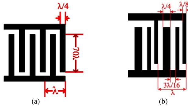
Fig. 1 – Bi-directional IDT (a) and SPUDT (b) configurations of the SAW strain sensor [16].
