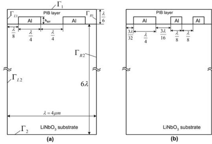
Fig. 2 – 2D unit cell structure employed in the FEM simulation, for bidirectional (a) and SPUDT (b) configurations of a SAW gas sensor.
