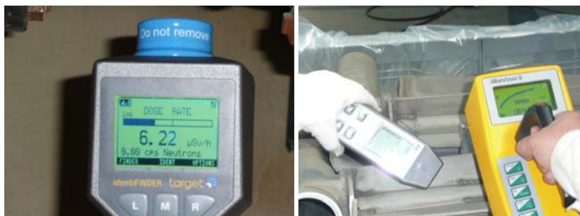
Fig. 1 – Portable dosimetric equipment – IDENTIFINDER, radiometer FH40G-L10 and MICROCONT.
