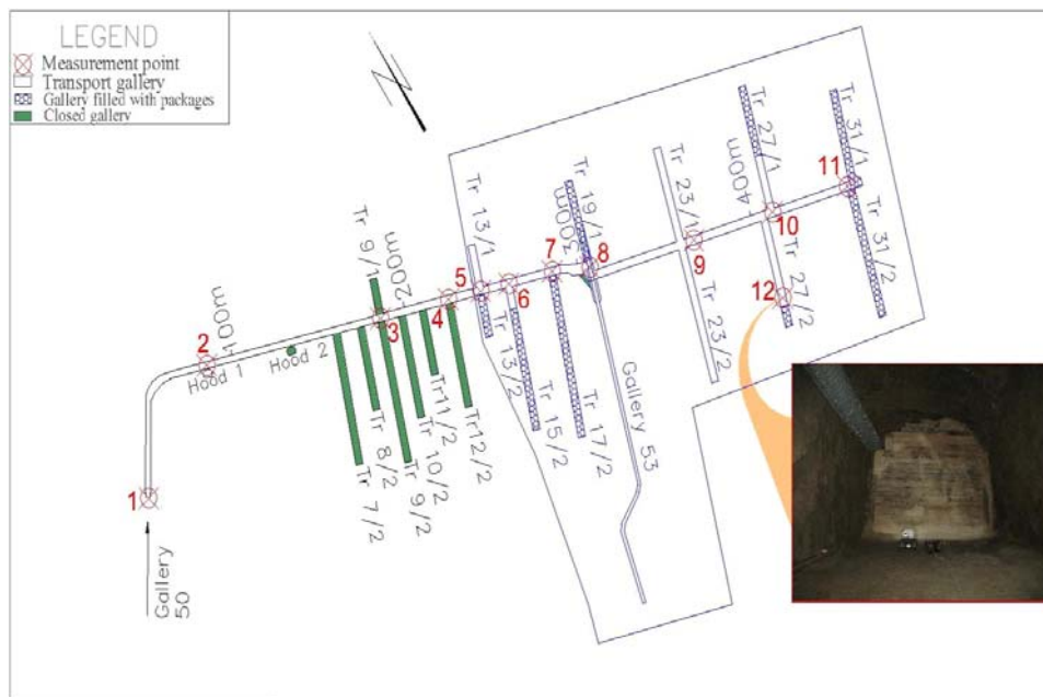
Fig. 1 – Location of the measurements points of the radon on the repository sketch.
