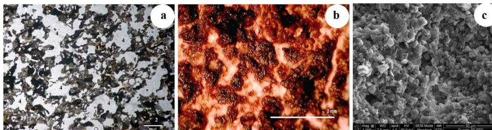
Fig. 2 – Sample A: a) Thin section: 1- bioclasts of benthic foraminifers, 2- fragments of red algae, 3- bioclasts of bryozoa, 4- secondary porosity, dissolution of the matrix, pore/ voids (The scale bare is 0,5mm); b) Alizarin Red S stained section: calcite red-orange /black coloured and dolomite uncoloured; c) SEM: voids and calcite crystals.
