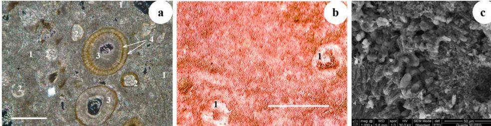
Fig. 4 – Sample C: a) Thin section: 1- sparite calcite, 2- bioclasts, 3-ooides, 4-iron hydroxides. The scale bare is 1mm. b) Alizarin Red S stained section: 1-poor content of ooides. The content of calcite is similar to that of the dolomite (percent of red/uncoloured zones are close). c) SEM: voids (right-down corner) and full core ooides (to the left corner).
