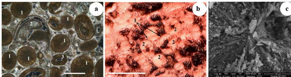
Fig. 3 – Sample B: a) Thin section of sample: 1- ooides, 2- bioclasts, 3- ooides wiht empty vortex, 3- sparitic mosaic calcite. The scale bare is 1mm; b) Alizarin Red S stained section: 1- sutural contact between ooides, 2- ooides (high number of empty or full ooides' cores); c) SEM: the core of one full ooid.
