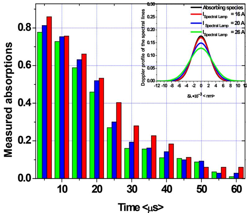
Fig. 6 – Temporal evolution of the absorption of the Neon line at 633.4 nm obtained during the temporal afterglow plasma of HCPD, measured using the pulsed spectral lamp at different peak currents (16 A – red, 20 A – blue, 26 A – green) (color online).
