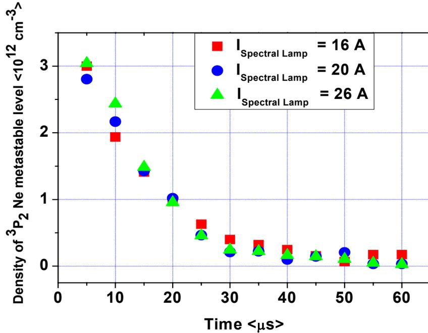
Fig. 8 – The temporal evolution of  $^3P_2$  Neon metastable level density in the temporal afterglow plasma according to the absorption measurements on  $^3P_2 - 2p^4$  transition at 633.4 nm.
