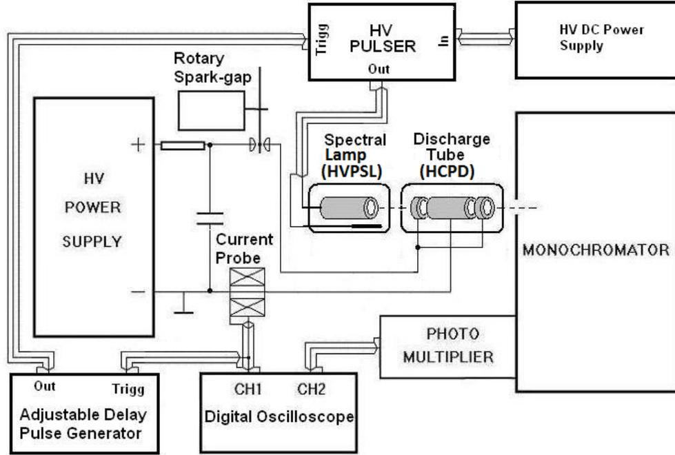
Fig. 1 – Experimental set-up for optical absorption measurements with temporal resolution using a pulsed hollow cathode spectral source.
