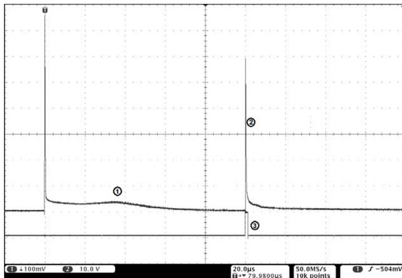
Fig. 3 – The Ne light signal at 633.4 nm; (1) Light emitted by the afterglow plasma of HCPD; (2) Light emitted by HVPSL and passing through HCPD; (3) Trigger signal from Adjustable Pulse Generator.
