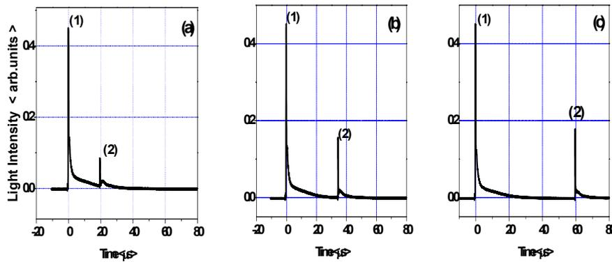
Fig. 4 – The Ne light signal at 633.4 nm; (1) Light emitted by the afterglow plasma of HCPD; (2) Light emitted by HVPSL and passing through HCPD at various temporal position; (a) 20 $\mu$ s, (b) 35 $\mu$ s and (c) 60 $\mu$ s.
