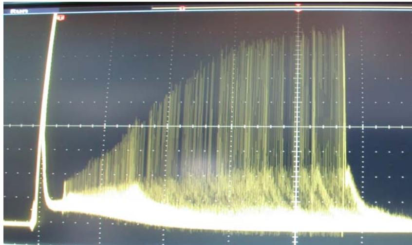
Fig. 5 – Photo representing the temporal evolution of the intensity of the light pulse emitted by the spectral lamp at 633.4 nm and passing through the temporal afterglow plasma of the discharge tube.
