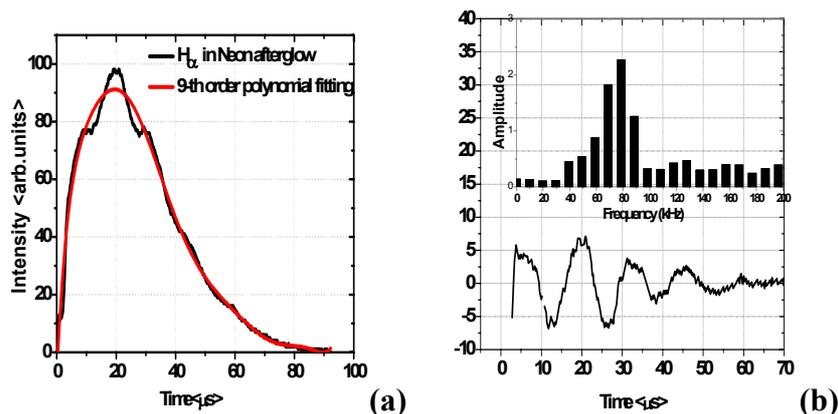
Fig. 2 – (a) The modulations of the  $H_{\alpha}$  line of hydrogen in the neon and the fitted curve, (b) the clean oscillations, and the Fourier spectrum of the oscillations.
