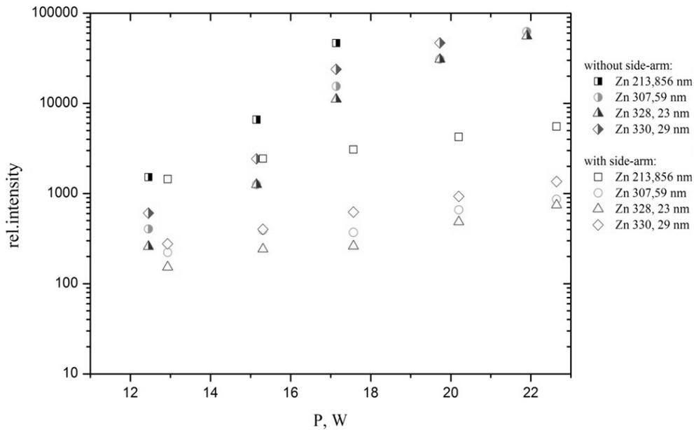
Fig. 8 – Intensities of several Zn spectral lines depending on power applied to generator in H-discharge mode.
