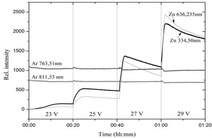
Fig. 4 – Stability of Zn and Ar spectral lines in HFEDL with side-arm.
