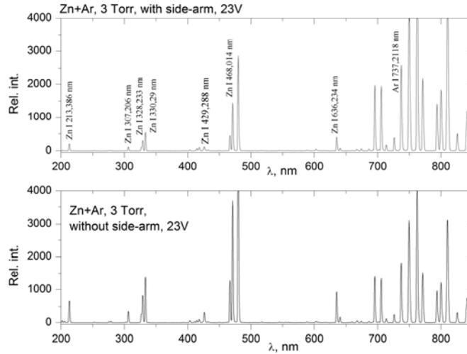
Fig. 6 – a) spectrum of Zn+Ar lamp with a side-arm, b) spectrum of lamp with-out sidearm.
