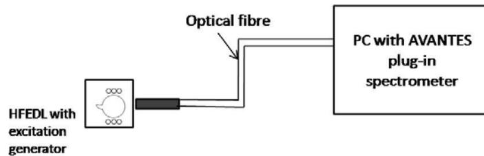
Fig. 2 – Experimental set-up for stability measurements with AVANTES spectrometer.
