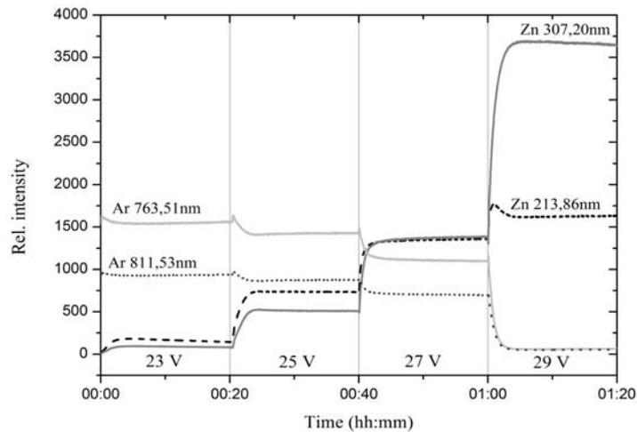
Fig. 5 – Stability of Zn and Ar spectral lines in HFEDL without side-arm.
