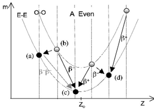
Fig. 2 – Illustration of a DBD process: nuclei (a) and (d) are stable against  $\beta$  decay, but unstable against  $\beta\beta$  decay:  $\beta^-\beta^-$  for (a) and  $\beta^+\beta^+$  for (d).
