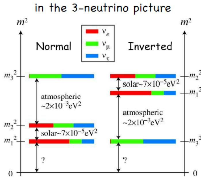
Fig. 1 – Hierarchical neutrino mass scheme: a) normal hierarchy; b) inverted hierarchy.
