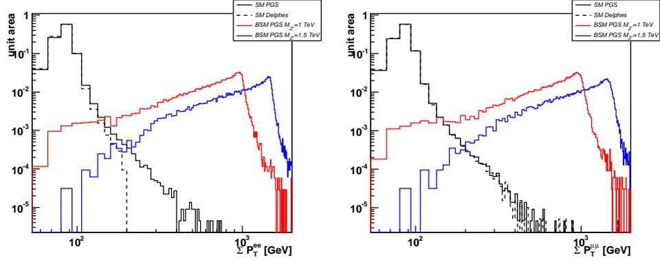
Fig. 5 – The scalar sum of transverse momenta  $P_T$  for dilepton final state (left: electrons, right: muons) is shown for the SM prediction using PGS and Delphes fast detector simulation and for  $Z'$  signal for 2 masses: 1 TeV and 1.5 TeV using PGS.
