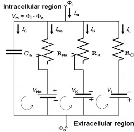
Fig. 1 – Linear and nonlinear elements in the membrane cell
