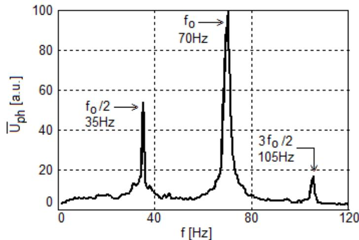
Fig. 6 – Spectrum of the lock-in amplifier output voltage near the upper bound of the first stability region. Experimental conditions:  $f_0 = 70\text{Hz}$ ,  $V_0 = 3.4\text{kV}$ ,  $U_x = 330\text{V}$ ,  $U_z = 920\text{V}$ . Experimental result.
