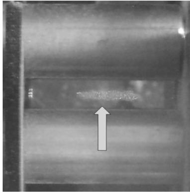
Fig. 2 – Microparticles cloud (pointed by the arrow) stored along the longitudinal axis of the linear trap [19].
