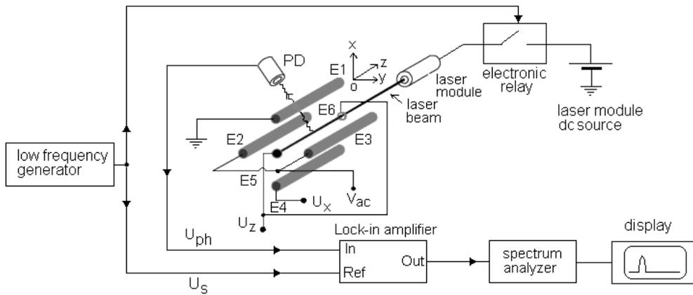
Fig. 3 – Block diagram of the measurement chain.
