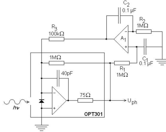
Fig. 4 – Electronic circuit of the photodetector [21].
