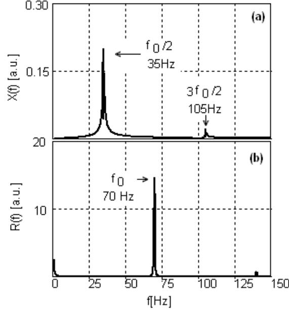
Fig. 5 – Fourier transform  $X(f)$  (a) and  $R(f)$  (b) of the rectangular  $x(t)$  and radial  $r(t)$  coordinates, respectively, for  $q_x = 0.908$ ,  $a_x = 0$ ,  $f_0 = \Omega/2\pi = 70\text{Hz}$ ,  $\delta = 0.01$ . Numerical result.
