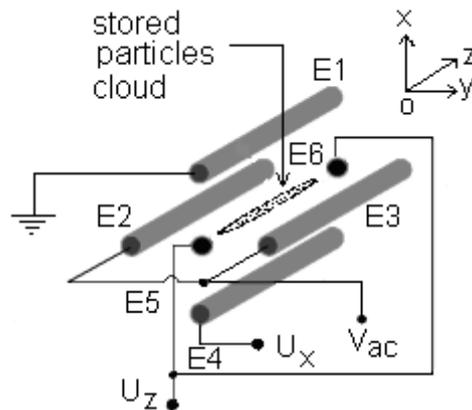
Fig. 1 – Spatial arrangement and electrical circuit of the electrodes for a linear electrodynamic trap.
