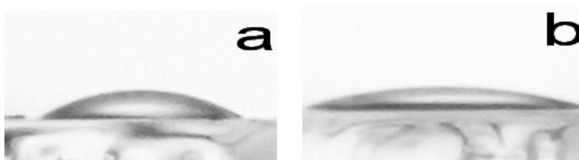
Fig. 6 – Water droplet on a not treated (a) and a 5 s He DBD treated (b) glass surface.
