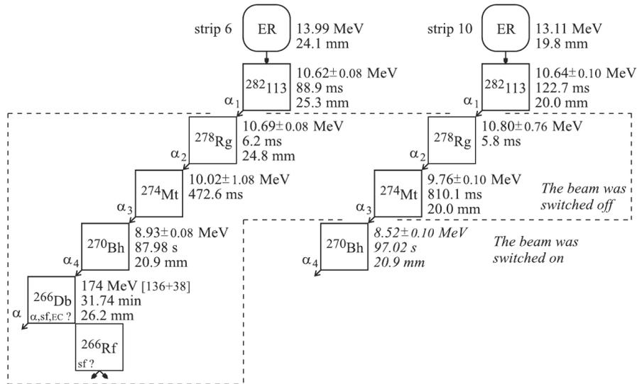
Fig. 2 – Time sequences in the decay chains of  $^{282}_{113}$  observed in the  $^{237}\text{Np} + ^{48}\text{Ca}$  reaction [5]. The measured  $\alpha$ -particle energies, decay times, and positions of the observed events with respect to the top of the focal-plane detectors are shown.
