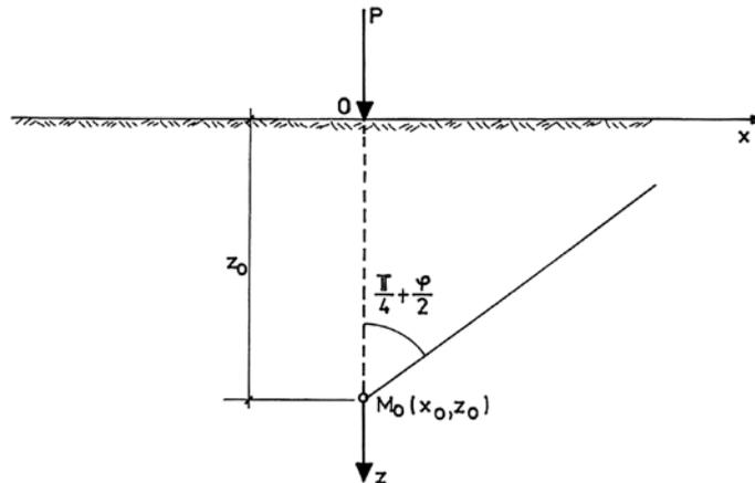
Fig. 2 – Finding out the point location at ultimate equilibrium and the direction of the planes of ultimate equilibrium cross through this point – situated on the vertical line of the application point of the focused force.
