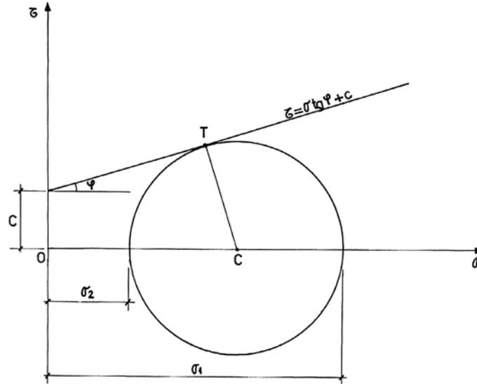
Fig. 1 – Graphical representation of the ultimate equilibrium for a point in an earth massif, in the hypothesis of a plane state of tensions.
