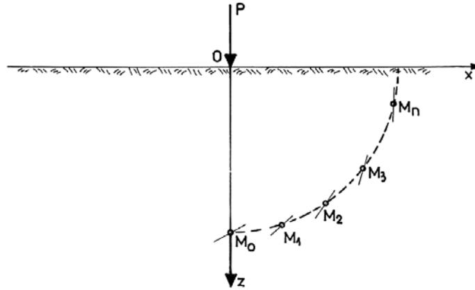
Fig. 4 – Construction of the breaking surface.
