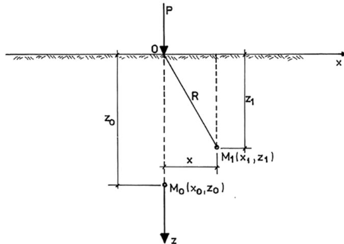
Fig. 3 – Finding out the position of a neighbouring point at ultimate equilibrium.
