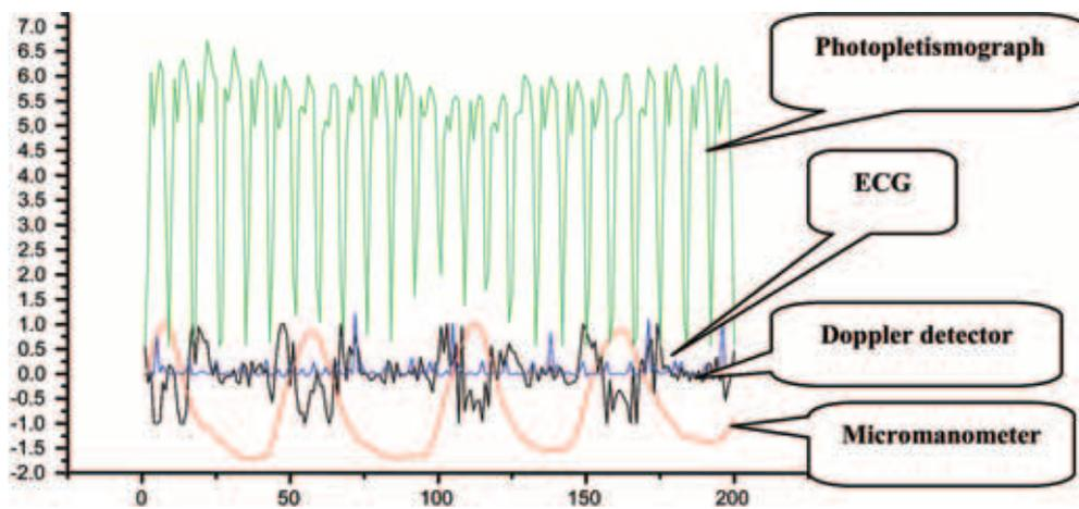
Fig. 2 – Cardio-respiratory activity monitored by ECG, Doppler effect, thorax transducer and photoplethysmograph.
