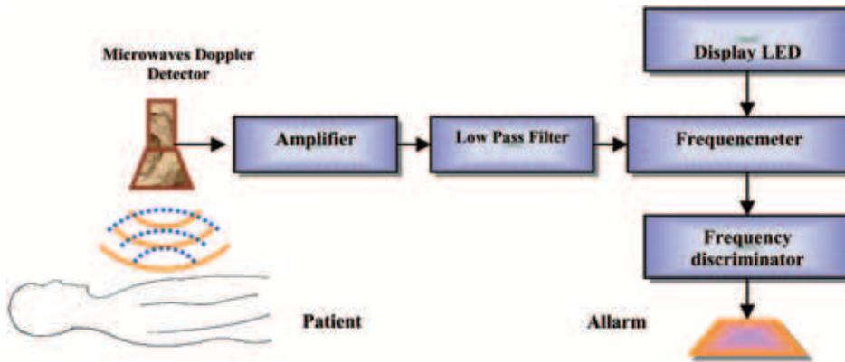
Fig. 6 – Bloc diagram for patient monitoring devices.
