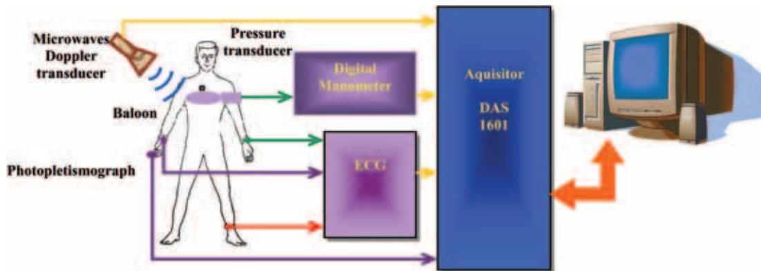
Fig. 1 – Experimental setup for the study of cardiorespiratory activity using a microwave Doppler transducer.
