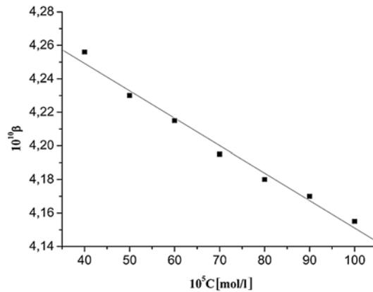
Fig. 4 – Adiabatic compressibility *versus* salt concentration.
