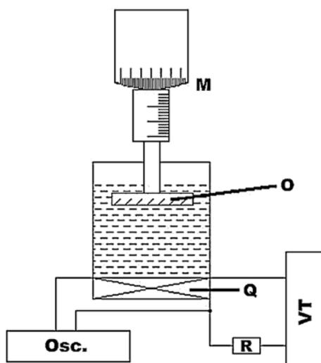
Fig. 1 – Ultra-acoustic interferometer.
