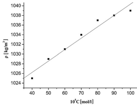
Fig. 3 – Density of ocular humours *versus* salt concentration.
