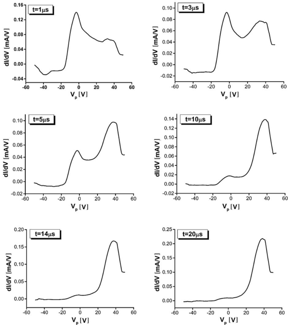
Fig. 3 – Electron energy distribution functions proportional with the first derivatives of the current-voltage characteristics of the Langmuir probe.
