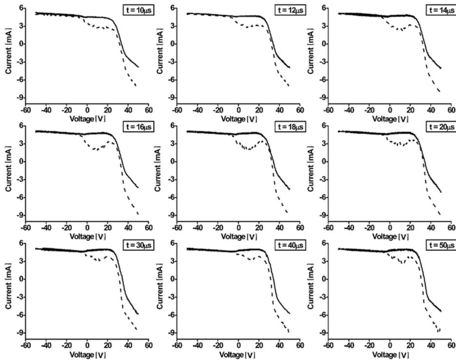
Fig. 2 – Current-voltage characteristics of the hot probe with both orientations of the probe (solid line correspond to the orientation of the probe toward the electrode, while the dashed line correspond to the orientation of the probe away from the electrode).
