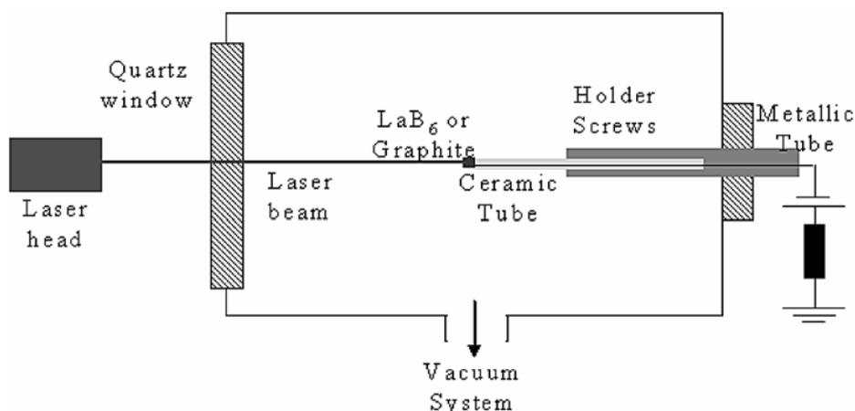
Fig. 1 – Schematic representation of the experimental set-up.
