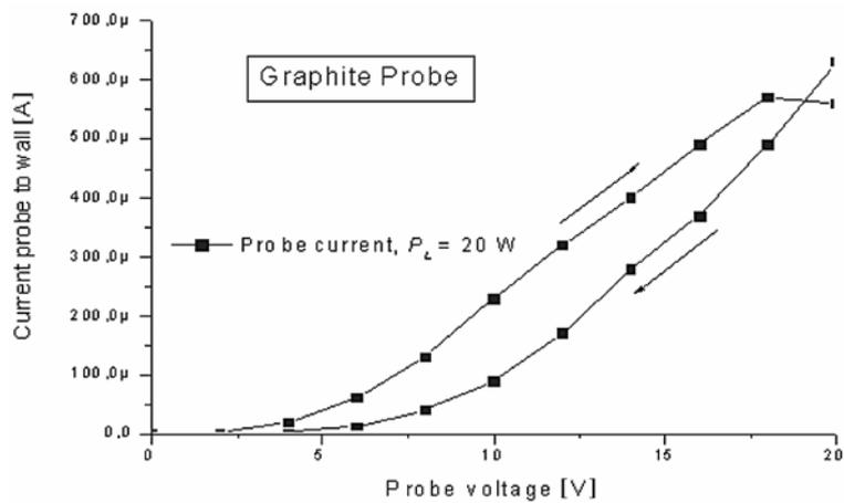
Fig. 5 – Current-voltage characteristic  $I_p(V_p)$  of the graphite probe for constant laser heating power.
