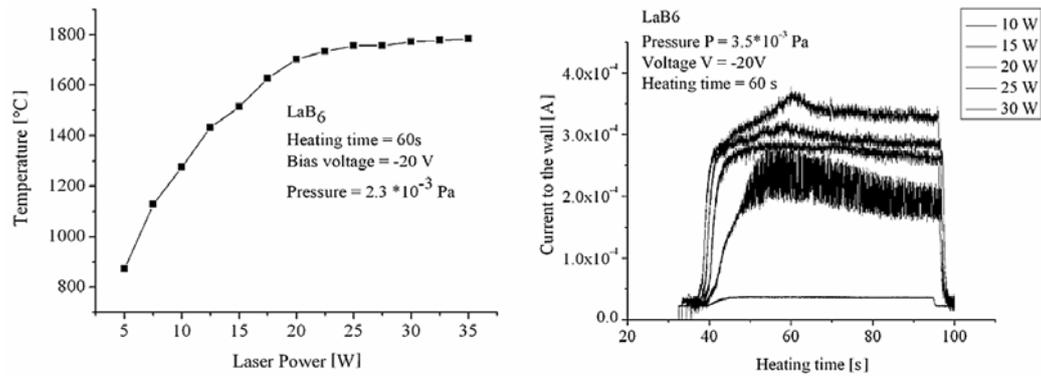
Fig. 4 – Temperature vs. laser power and current to test chamber wall vs. time for LaB<sub>6</sub> laser heated emissive probe. The exposure time (heating time) was 60 seconds and the applied potential on the probe was  $V = -20$  V.
