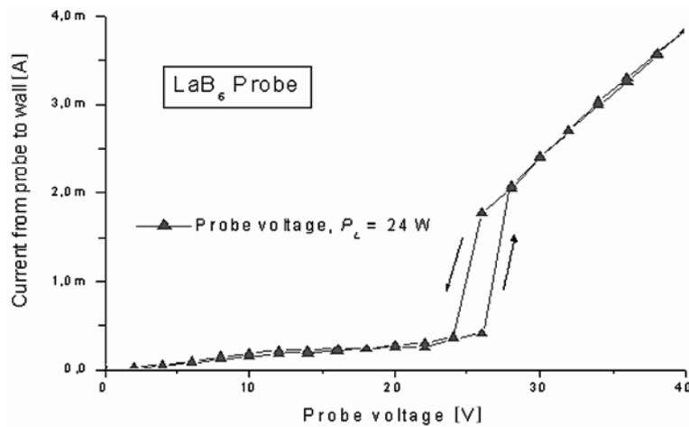
Fig. 6 – Current-voltage characteristic  $I_p(V_p)$  of the  $\text{LaB}_6$  probe for constant laser heating power.
