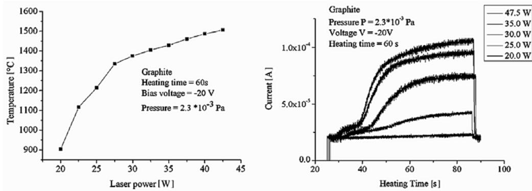
Fig. 3 – Temperature vs. laser power and current to test chamber wall vs. time for graphite laser heated emissive probe. The exposure time (heating time) was 60 seconds and the applied potential on the probe was  $V = -20$  V.
