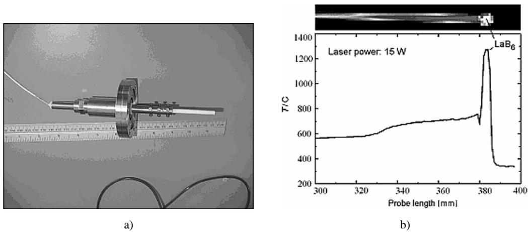
Fig. 2 – (a) Probe design; (b) Temperature distribution in along probe ceramic shaft obtained with an infrared camera.
