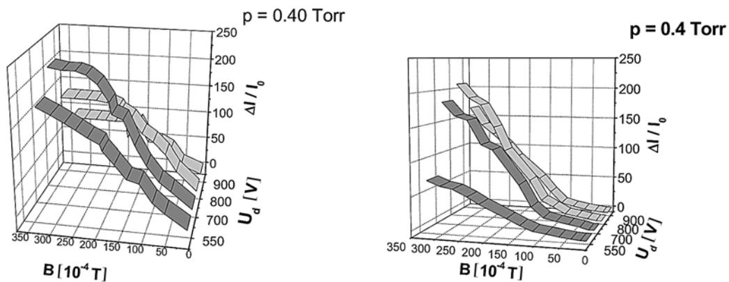
Fig. 2 – The relative variation of the TVI ( $\Delta I/I_0$ ) versus magnetic field ( $B$ ) for different values of discharge potential ( $U$ ) in the two configurations: a) CMC (central electrode cathode) and b) ICMC (central electrode anode).
