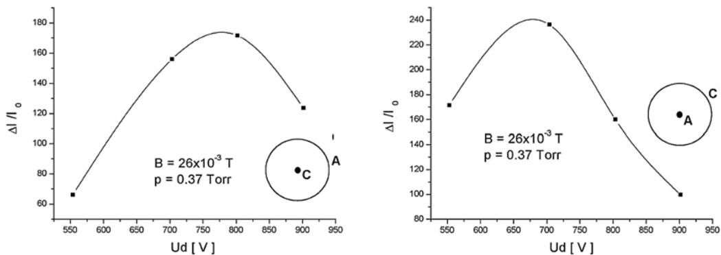
Fig. 3 – The dependence  $\Delta I/I_0$  versus  $U$  in the two discharge configurations: a) CMC and b) ICMC.
