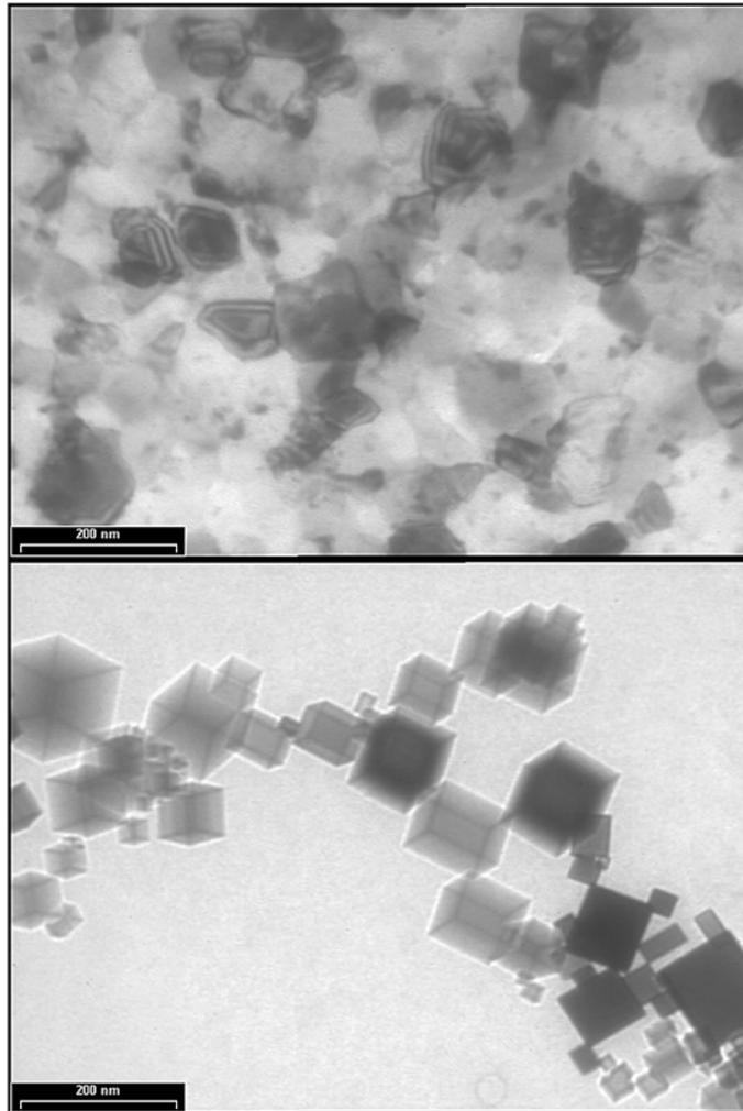
Fig. 1 – BF-TEM image of aluminum film and MgO nano-sized crystal.
