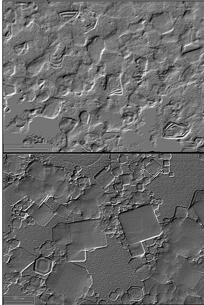
Fig. 2 – Processed BF-TEM image of aluminum film and MgO nano-sized crystal using shadow filter to improve contrast of particle.
