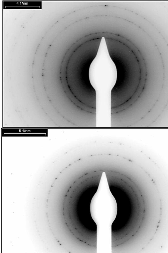
Fig. 4 – SAED image used for evaluate mean diameter. First interior ring in both images represent (111) reflection used in Scherrer equation to evaluate mean diameter.
