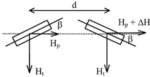
Fig. 2 – The measuring error due to the transversal field.
