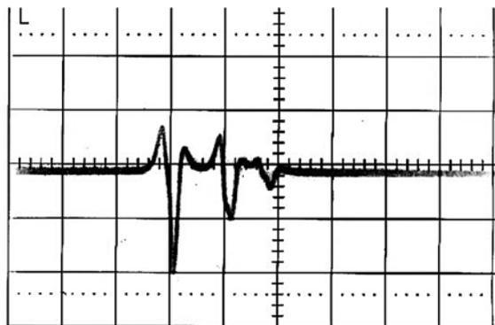
Fig. 4 – The gradient signal produced by the passage of three bodies of different sizes.
