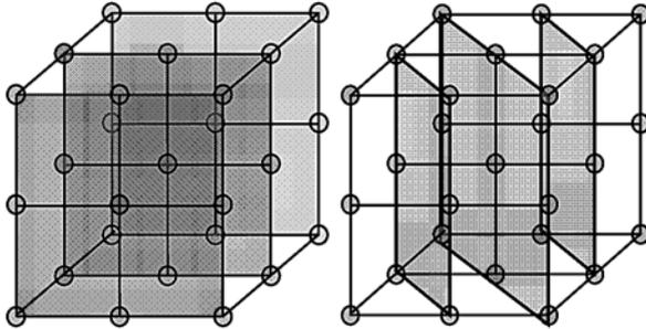
Fig. 3 – The crystalline lattice of NaCl – planes 100 and 110.
