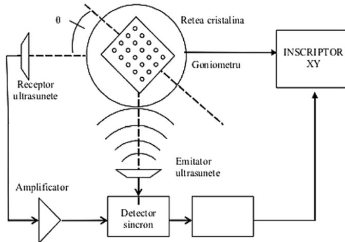
Fig. 2 – The experimental setup for rotating method.
