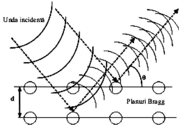
Fig. 1 – Ultrasonic waves diffraction.
