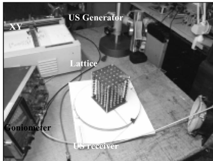
Fig. 4 – The experimental installation for the study of diffraction using the rotating method.
