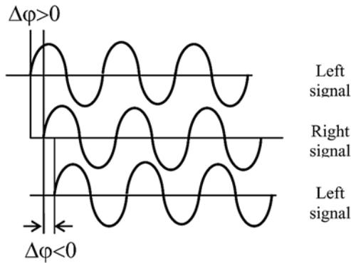
Fig. 6 – Phase difference between the two channels.
