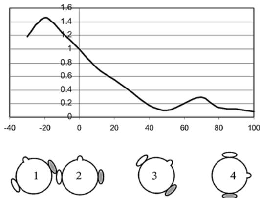
The diagram from Fig. 7 shows the dependence of the amplitude of the sound source function of the position of right ear for a 10 kHz frequency. Turning the head on the left is noticed the growth of the intensity of the sound further to an angle of 20 degrees, due to the fact that the ear has got closer to the sonorous source. Because the experiment was not made in an aneroïdal room, the experimental results are easy influenced by minor reflexion and interferences.
