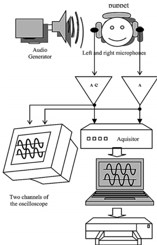
Fig. 4 – Block diagram of the experimental setup for acoustic perception.
