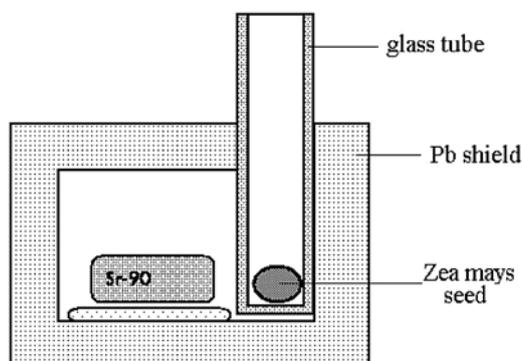
Fig. 1 – The beta-irradiation chamber.
