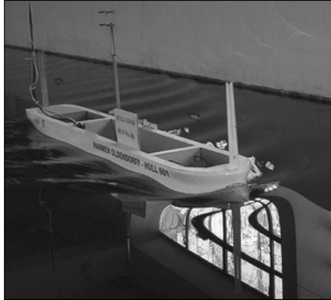
Fig. 5 – Wave pattern at full load, v_s = 16.57 Kn.
