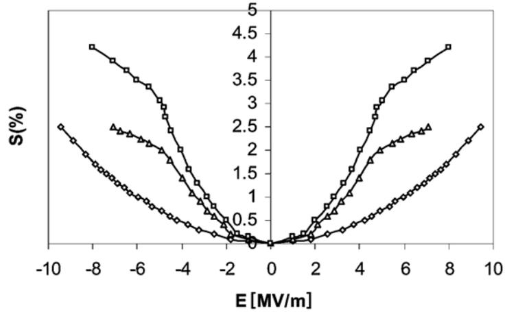
Fig. 1 – Dependence of strain on electric field:  $\diamond$  – sample 1;  $\square$  – sample 4;  $\Delta$  – sample 5 (Table 1).
