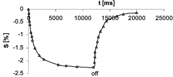
Fig. 4 – Time response of contraction and relaxation processes in sample 5 at 5.4 MV/m.
