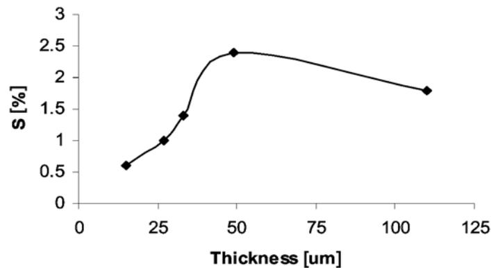
Fig. 2 – Thickness dependence of the induced strain for 4.5 MV/m.
