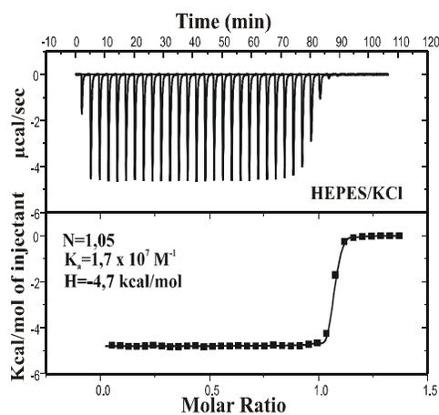
Fig. 3. The thermogram (up) and the titration isotherm (down) of a 5 mM  $\text{CaCl}_2$  solution in 1.4 ml 0.5  $\mu\text{M}$  EDTA solution, in 50 mM HEPES/100 mM KCl, at pH 7.4 and 30  $^\circ\text{C}$ .
