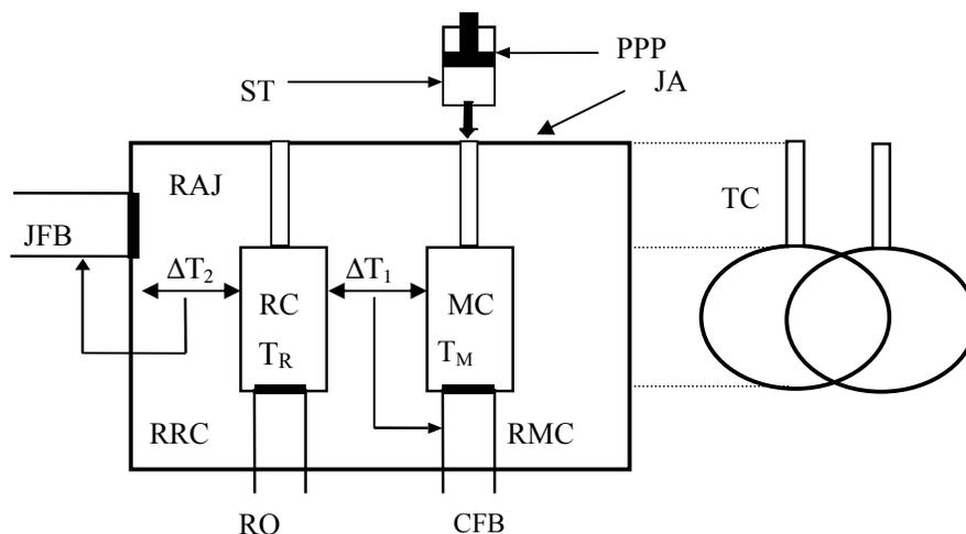
Fig. 1. The simplified schema of ITC calorimeter.
