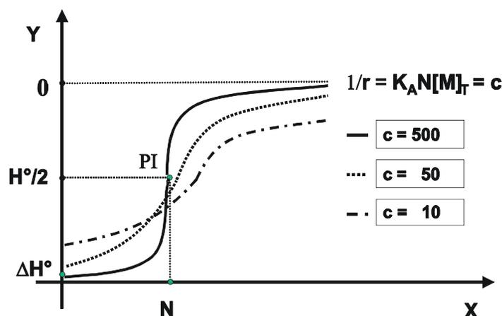
Fig. 2. Binding isotherms for different values of  $c$  parameter.
