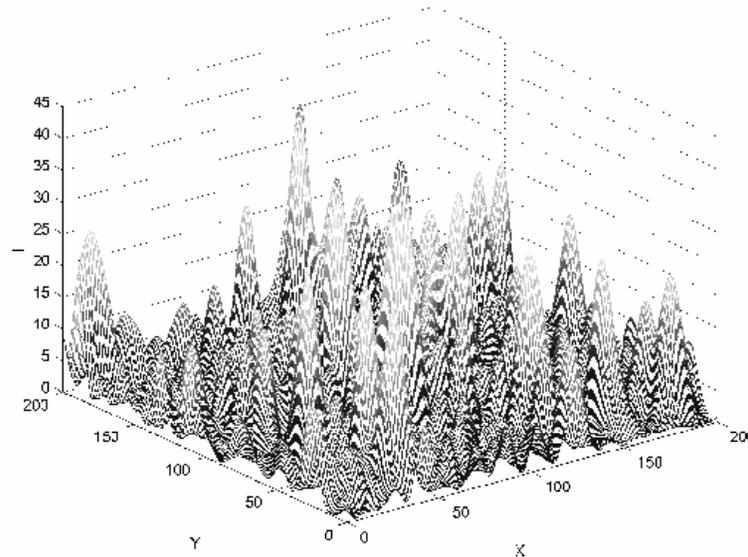
Fig. 2. Light intensity distribution on the screen, for a sample with 50 scattering centres.
