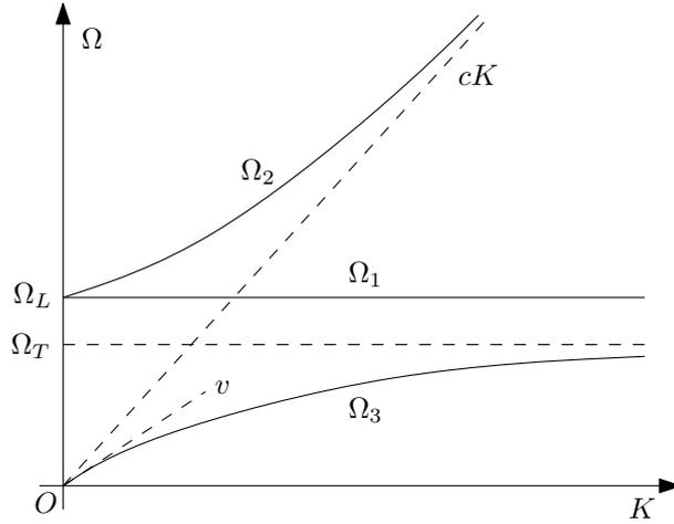
Figure 1 – The polarization longitudinal eigenmode  $\Omega_1$  and the two transverse eigenmodes  $\Omega_{2,3}$ . We note the velocity  $v$  of the "renormalized" transverse waves ( $cK$  is the frequency of the free transverse waves).
